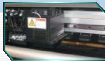
Precision Rail & Carriage, to provide accurate placement of dots.
